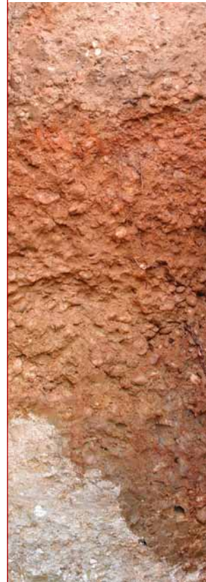
Gravel on clay subsoil
